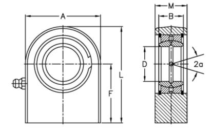
= 123 Α a (degrees) = 6 В = 35 D = 50 Dynamic load C (kN) = 156F = 88 L = 149.5
